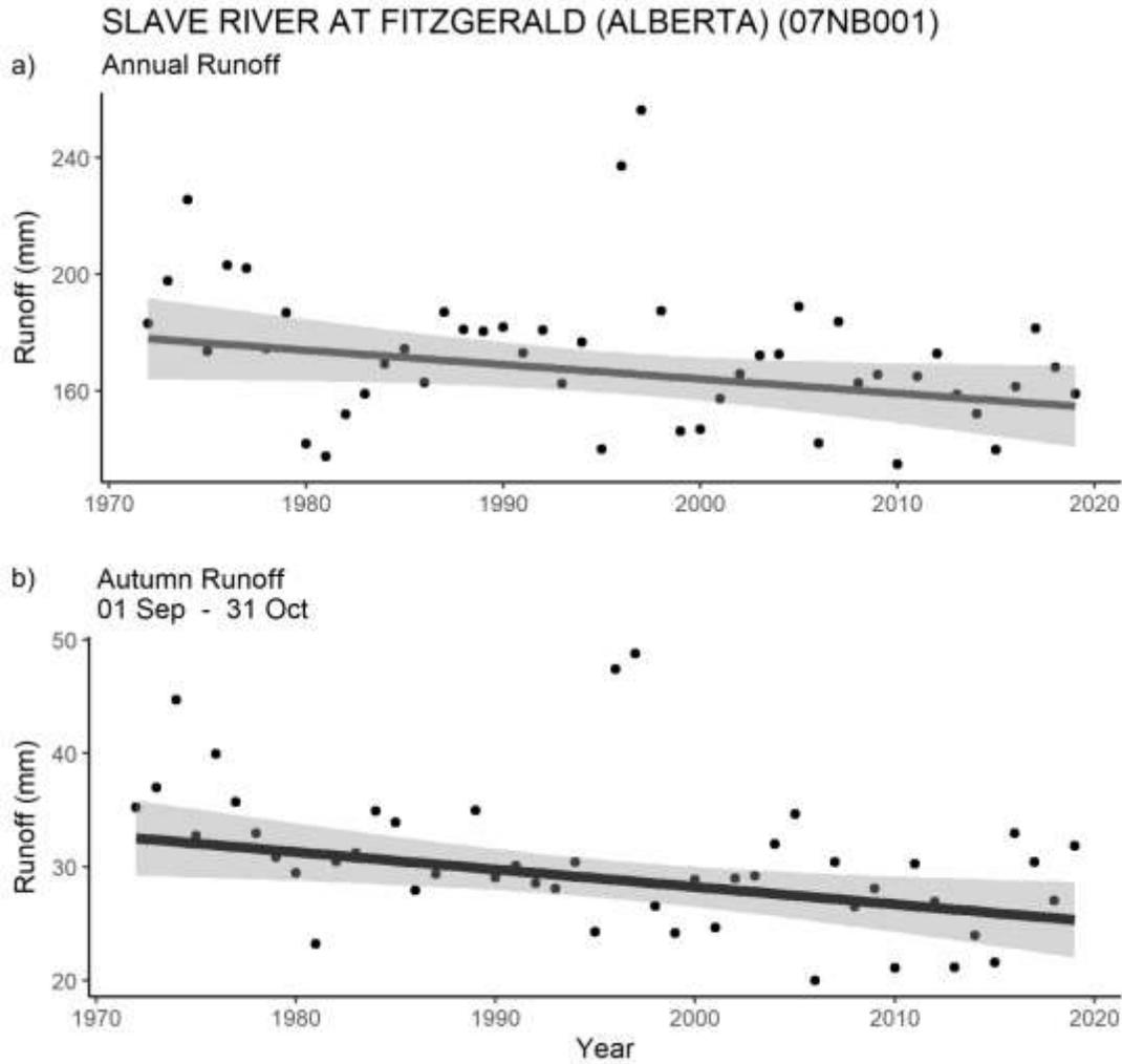
**Figure 8:** Trend analysis of annual runoff (mm) and autumn runoff (mm) for the Slave River, using the Mann-Kendall trend test, WSC data 1972 to 2019; a) trend line indicates statistically significant decrease in annual runoff volume (grey:  $p < 0.05$ ); b) trend line indicates statistically significant decrease in runoff volume for September and October (black:  $p < 0.01$ ).
