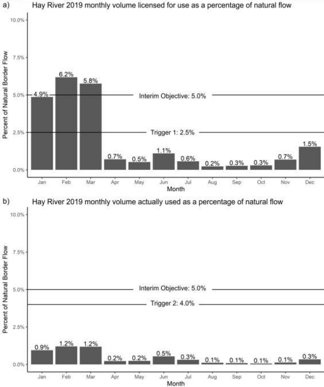
**Figure 6:** a) Trigger 1: Hay River 2019 monthly allocation as percentage of natural flow; b) Trigger 2: Hay River 2019 monthly use estimate as percentage of natural flow
