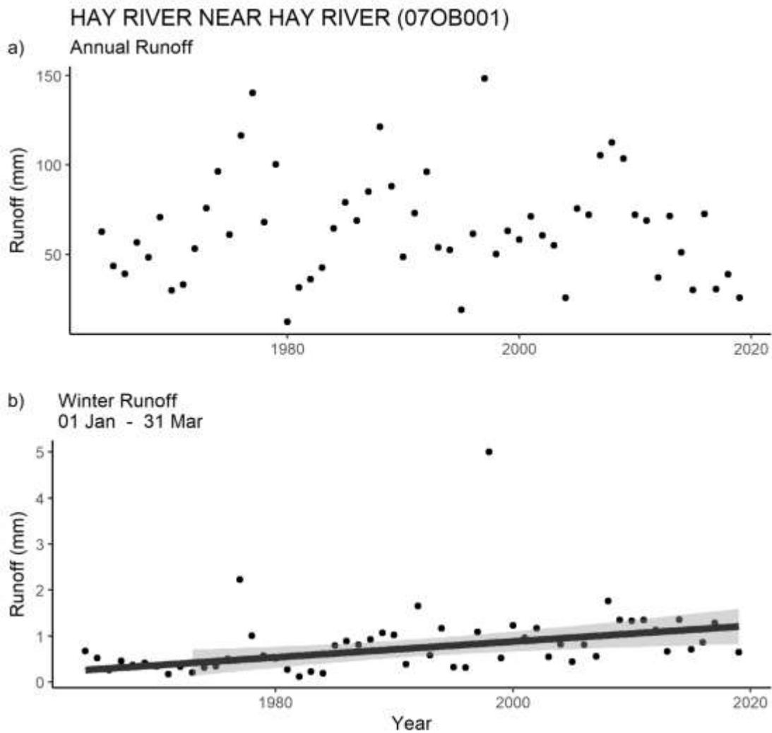
**Figure 2:** Trend analysis of annual runoff (mm) and winter runoff (mm; 01 Jan to 31 Mar) for the Hay River, using the Mann-Kendall trend test, WSC data 1963 to 2019; a) no statistically significant change in annual runoff volume (grey:  $p > 0.05$ ); b) statistically significant increases in winter runoff ( $p < 0.01$ ).
