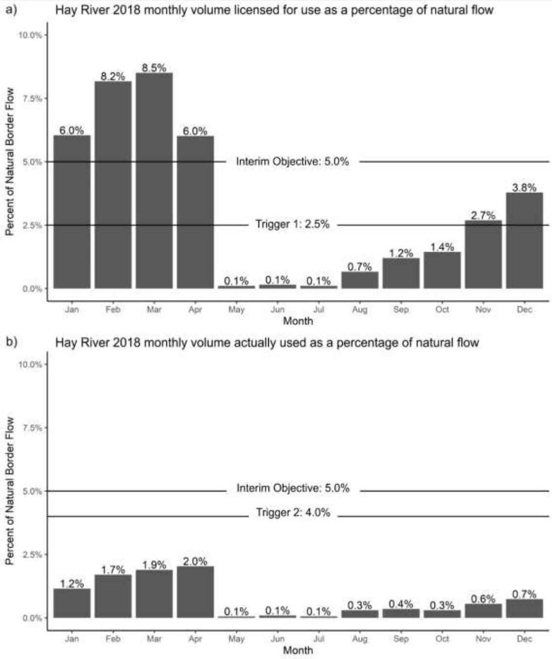
**Figure 5:** a) Trigger 1: Hay River 2018 monthly allocation as percentage of natural flow; b) Trigger 2: Hay River 2018 monthly use estimate as percentage of natural flow
