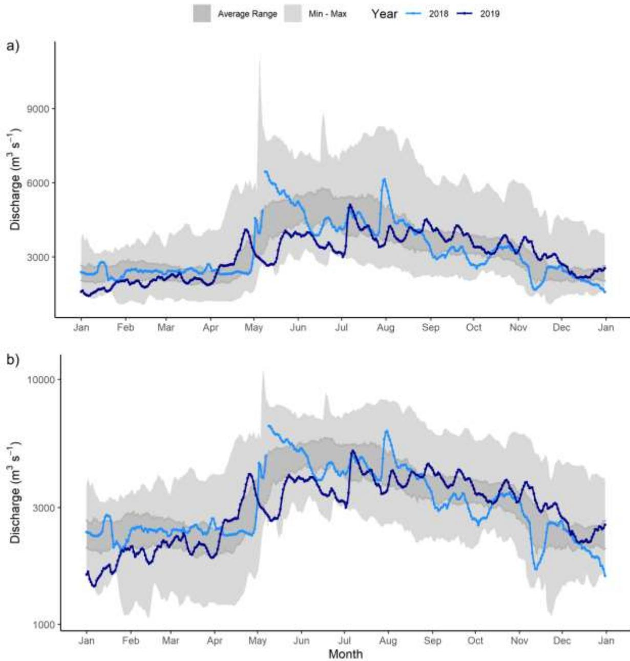
**Figure 10:** Slave River discharge for the years 2018 and 2019 relative to the historic average range (depicted as the interquartile range), and minimum and maximums on: a) linear scale y-axis; and b) log scale y-axis
