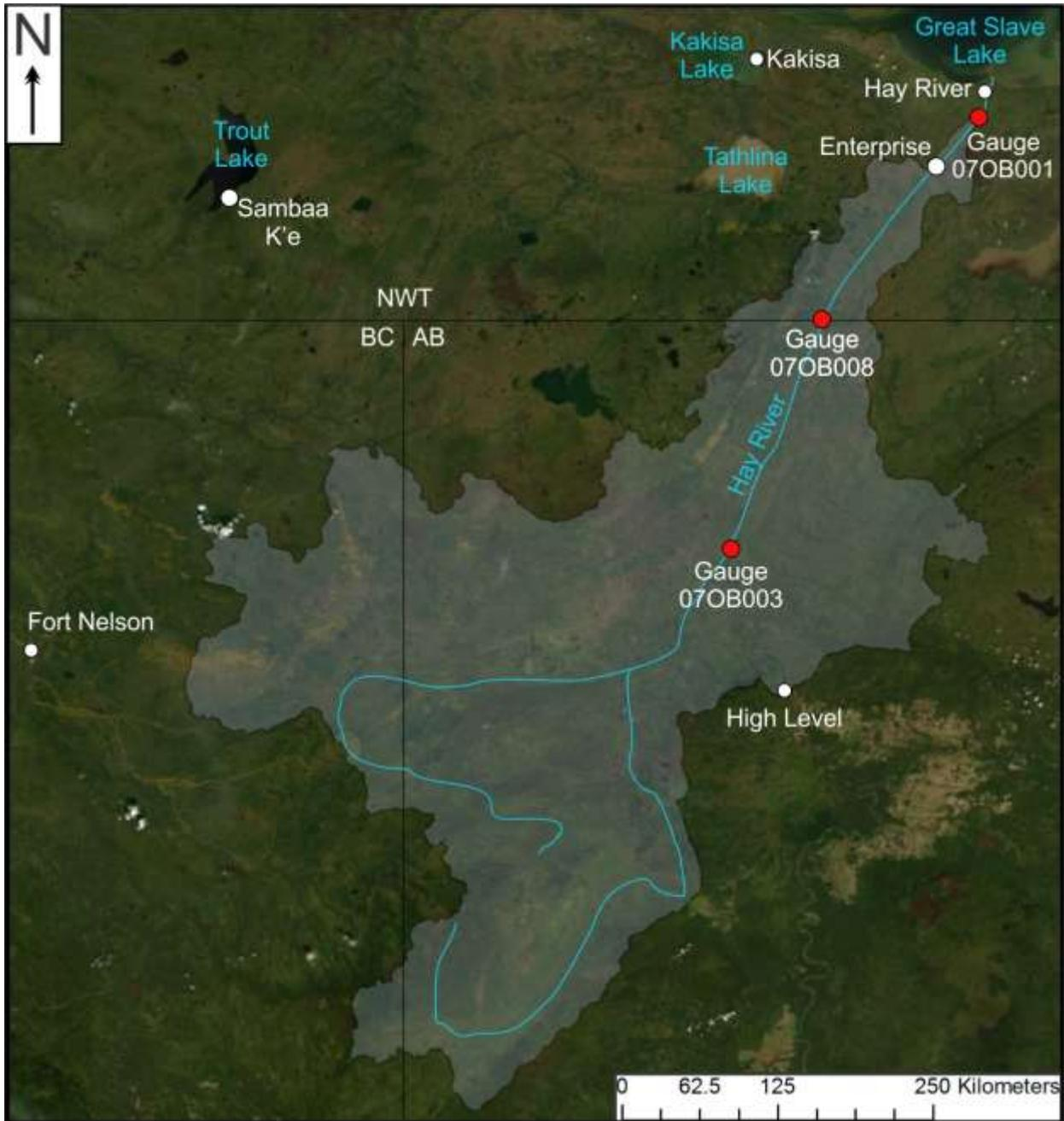
**Figure 1:** Map of the Hay River basin, including Water Survey of Canada hydrometric gauges on the Hay River. Note that the superimposed renderings of the river network are for illustrative purposes only.
