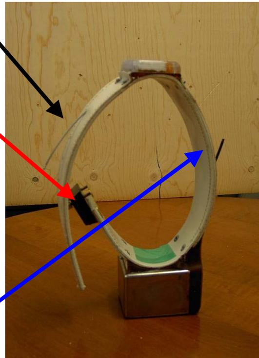
Figure 2. Telonics TGW-3680 GPS collar standard design with release mechanism (red arrow), satellite beacon (blue arrow), VHF beacon (black arrow) and a GPS antenna (top of collar).
