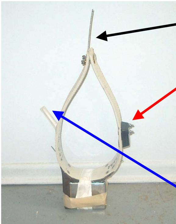
Figure 1. Telonics ST-20 satellite collar teardrop design with release mechanism (red arrow), satellite beacon (blue arrow) and VHF beacon (black arrow).
