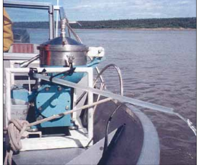
The centrifuge is a large sampler that separates the river water from the suspended sediment. This is important because the water and suspended sediments of the Peel River can have very different chemistry. We want to look at both separately.
