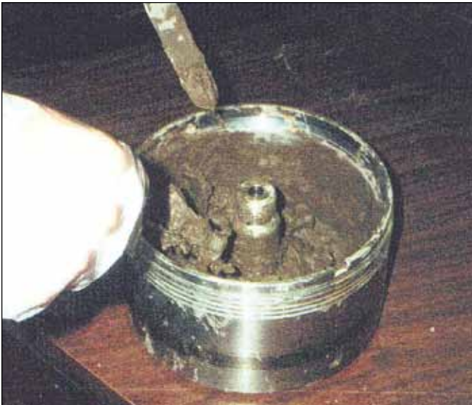
The suspended sediment is collected in the centrifuge bowl, transferred into sampling jars and sent to the laboratory for analysis.
