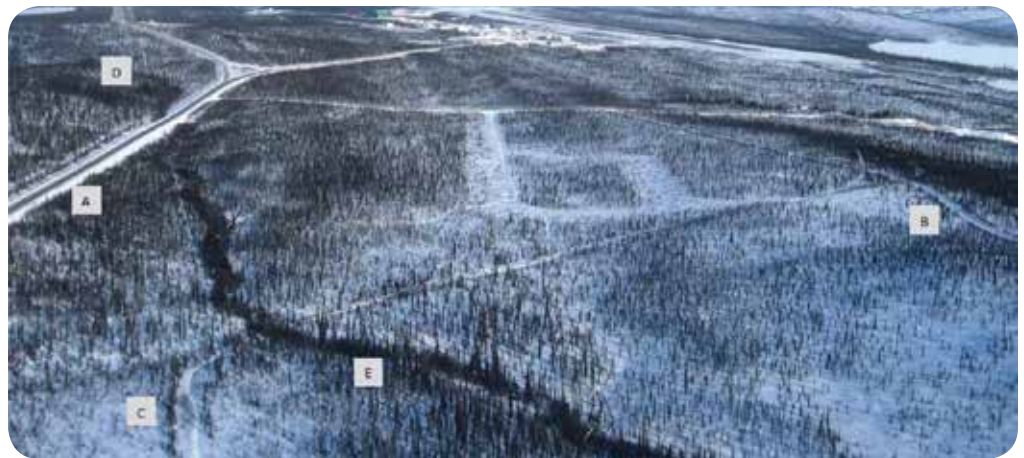
Fig. 1. A variety of linear developments common in northern regions; (A) an all-season road, (B) a snow road, (C) a winter trail, and (D) seismic line. These types of linear developments often cross watercourses, such as the creek (E), and could impact fish and fish habitat if not constructed and maintained properly. The Inuvik Airport is shown in the background, near the Town of Inuvik, NWT, Canada. Photo: J. Kanigan, GNWT-ENR(CIMP).
