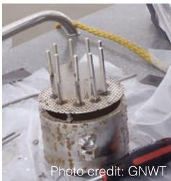
**PMDs (Polyethylene Membrane Devices)** are passive samplers that stay in the water for one month, up to 4 times per summer, to measure oil and gas-related chemicals (hydrocarbons) dissolved in the water. PMDs act like
