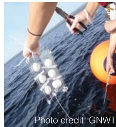
**Diffusion Gradients in Thin-Films passive samplers (DGTs)** act like sponges and pick up the toxic portion of dissolved metals in the water. DGTs are left in the water for 3 to 4 days. DGTs measure the concentrations of dissolved
