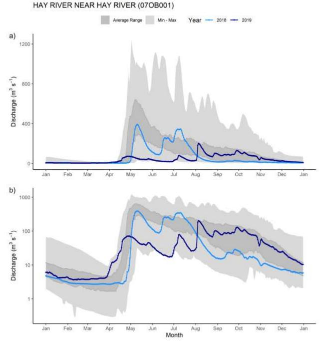
**Figure 4:** Hay River discharge for the years 2018 and 2019 relative to the historic average range (depicted as the interquartile range), and minimum and maximums on: a) linear scale y-axis; and b) log scale y-axis
