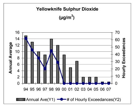
Figure 7 shows the general trends in SO<sub>2</sub> levels measured in Yellowknife air from 1994 to 2007. The bars track the annual average and the line shows the number of times in each year that the NWT 1-hour standard was exceeded. As illustrated by the graph, the number of exceedances has fallen to zero since the closure of Giant Mine in 1999.
