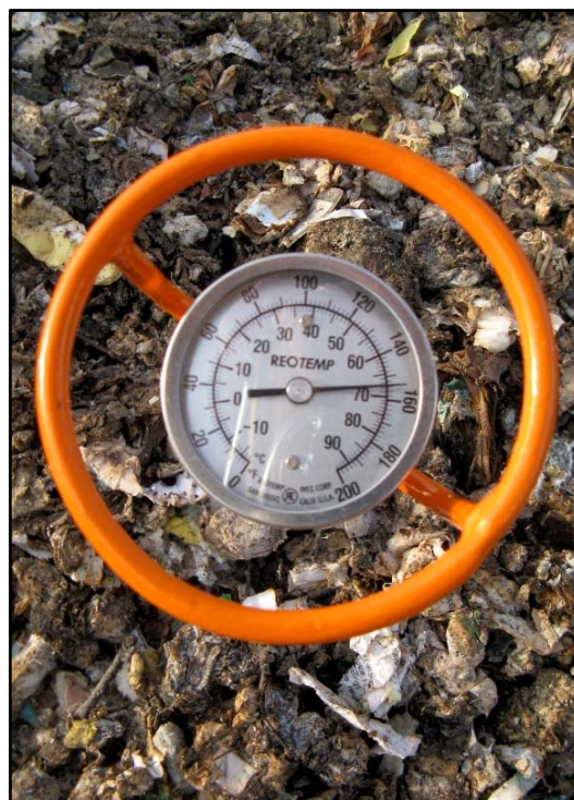
Composting windrow reaching 67°C
