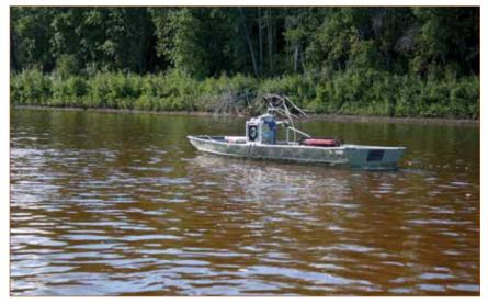
Centrifuge equipment mounted on boat anchored in the river. Centrifuge runs for up to 24 hours and collects the suspended sediment from the river. Both the suspended sediment and water are analyzed for many different substances, including metals and hydrocarbons.
