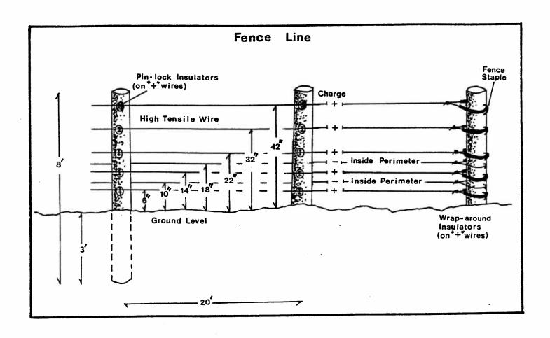
Figure 2. Design of the electric fenceline at the Norman Wells dump.
