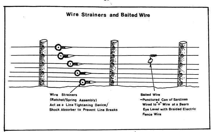
Figure 5. Wire strainer and bait location along the electric fence at the Norman Wells dump.
