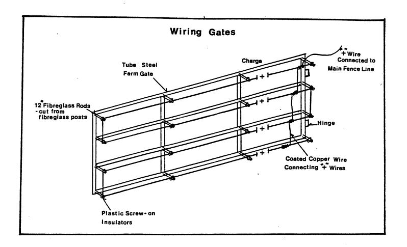
Figure 8. Design of gates and gate electric wiring for the electric fence at the Norman Wells dump.
