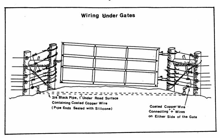
Figure 4. Design of the entrance and exit gates along the electric fence at the Norman Wells dump.
