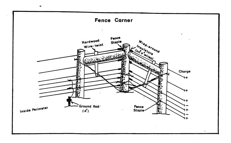
Figure 3. Design of corners along the electric fence at the Norman Wells dump.
