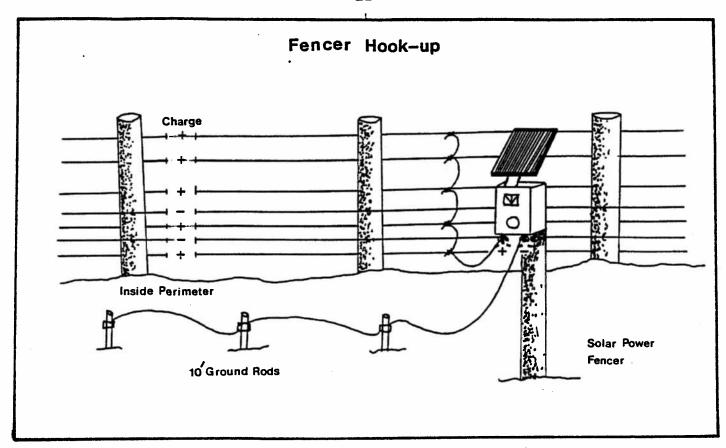
Figure 7. Mounting and grounding of the solar powered generator at the Norman Wells dump.
