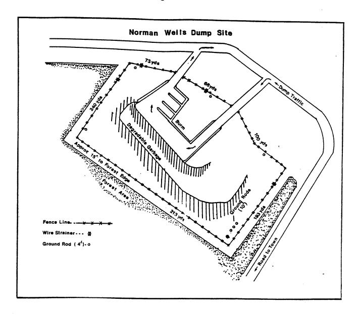
Figure 1. Entrance and exit points and the garbage disposal area within the electric fence at the Norman Wells dump.
