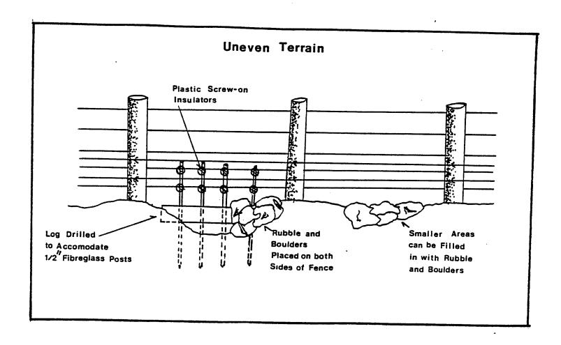
Figure 6. Infill of uneven areas under the electric fence at the Norman Wells dump.
