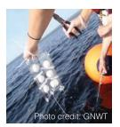
Diffusion Gradients in Thin-Films passive samplers (DGTs) act like sponges and pick up the toxic portion of dissolved metals in the water. DGTs are left in the water for 3 to 4 days. DGTs measure the concentrations of dissolved
