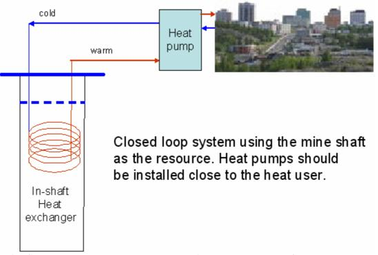
Fig. 2 – Closed loop geothermal development using the Robertson shaft as the resource. The heat exchanger (consisting of closed plastic tubing) is permanently installed in the shaft (below the water level).
