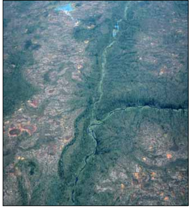
Better black and white spruce growth occurs along stream channels, where slopes are well drained and permafrost is not as close to the surface as it is on the adjacent uplands dominated by a complex of wet peat plateaus with small collapse scars and open black spruce forests.
